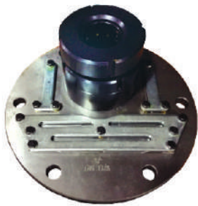
GAS VALVE COMPONENTS (AIR COMPRESSOR)
